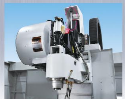
Counterweight air cylinder • Head housing moves up & down by air cylinder mounted in center of housing to reduce over load when Z axis moving up .
