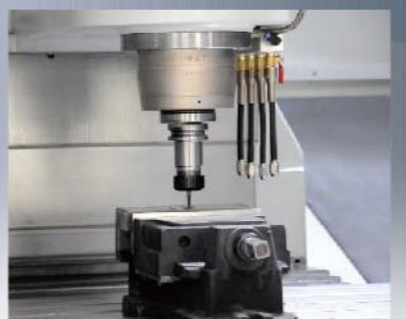
Rigid tapping test • It is necessary to do rigid tap test before make shipment. Tapping range : 3, 4, 5, 6mm
