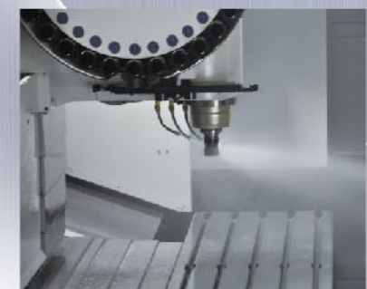
Coolant leak test • Coolant leak test for each machine before shipment.
