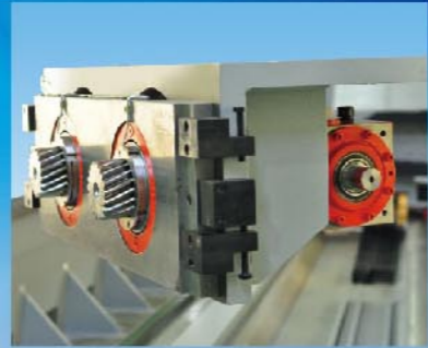
Dual gear box, pinion & installation
