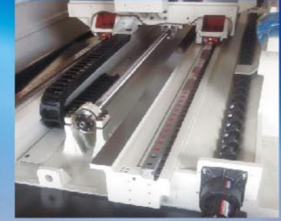
X axis with ball screw (TCM-266/286/366/386 & All TCM-344 model)
