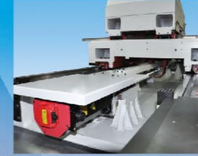
X axis ball screw • X axis ball screw assembly is with protected chip cover.
