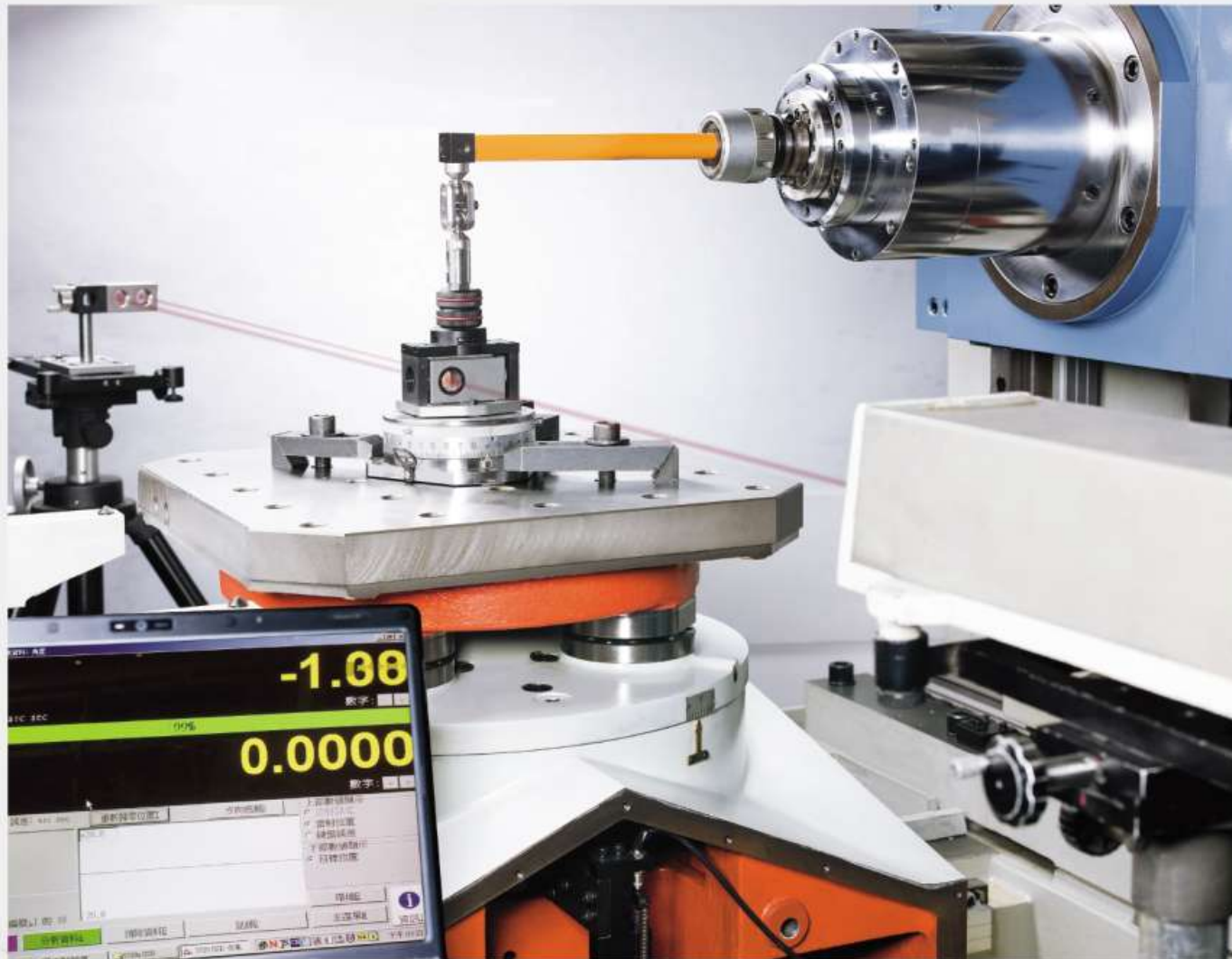
» Laser interferometer angular dividing accuracy measurement.
