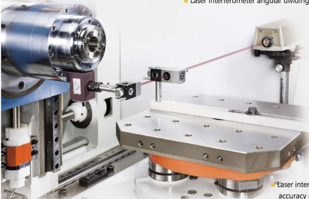
» Laser interferometer angular dividing accuracy measurement.
