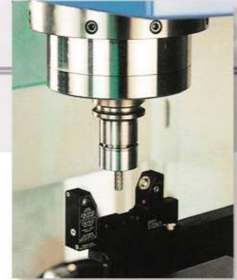
Non-Contact Type The laser tool length measuring device is used for detecting the tool wear condition while assuring machine accuracy at all times.
