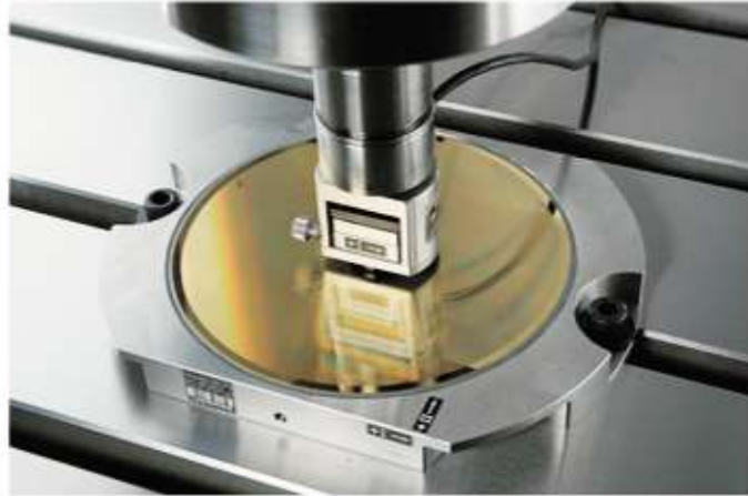
Grid Encoder Test To assure outstanding two-dimensional contour accuracy
