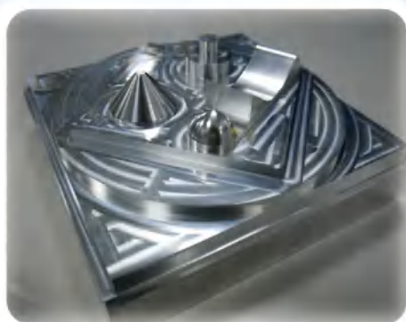
TAKUMI Test cutting workpiece Material: Aluminum 7075 Application: Surface / acute angle / positioning precision excellent performance
