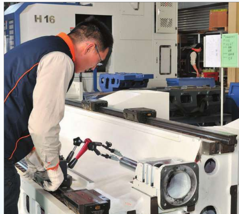
• Scrapping calibrated by the test bar All of the main assembling surfaces are hand scraped to optimize machine accuracy.
