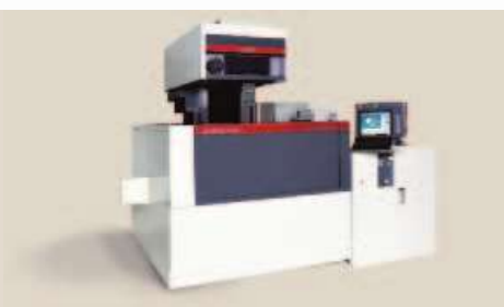
FA30-S Advance Travel paths X/Y/Z mm: 750 x 500 x 410 (420*) Overall dimensions of the machine W x D x H mm: 3495 (3732*) x 3143 x 2633 (2783*) Max. workpiece dimensions W x D x H mm: 1300 x 1000 x 405 (600*) * = V+ version for workpieces upto 600mm height
