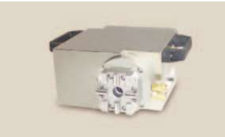
Rotation axis (B axis) Hirschmann H80RNCMI.6 This fully servo-controlled B axis allows wire eroding on a rotating, guided workpiece. Basic specification: Dimension (WxDxH): approx. 230 x 220 x 130 mm Axis centre above zero: 65 mm Indexing accuracy: +/- 5" Dead weight: approx. 35 kg Max. workpiece weight: 25 kg
