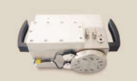
Rotation axis (B axis) Jauch Schmider R-10120D--060 This fully servo-controlled B axis also allows wire eroding on a rotating, guided workpiece. Basic specification: Dimension (WxDxH): 346 x 188 x 150 mm Axis centre above zero: 60 mm Indexing accuracy: +/- 5" Dead weight: approx. 30 kg Max. workpiece weight: 30 kg
