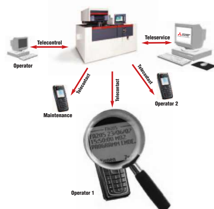
Telecontrol: Remote control via PC. Telecontrol realises the remote monitoring and remote control of the machine from any site. The optimisation of running processes is also possible.
