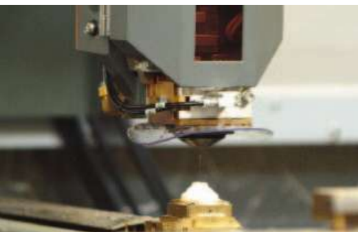
Threaded in 10 seconds: the AT system The combination of a new measuring sensor and a fast retract function gives you highest reliability and ultimate speed, even for smallest starting holes.
