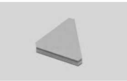
Innovative PCD processing that prevents unplanned material erosion Material: PCD grain size 10 \mu\text{m} Cutting height: 3 mm Wire electrode: 0.25 mm brass Surface quality: Ra 1.65 \mu\text{m}
