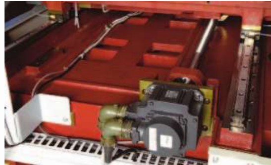
Direct drive and generously dimensioned spindles. The digital AC direct drive system, gives a shaft resolution of 0.05 µm. The spindle is also arranged exactly in the centre of the load in order to ensure "soft" axis movement. 10 years warranty on positioning accuracy is included.
