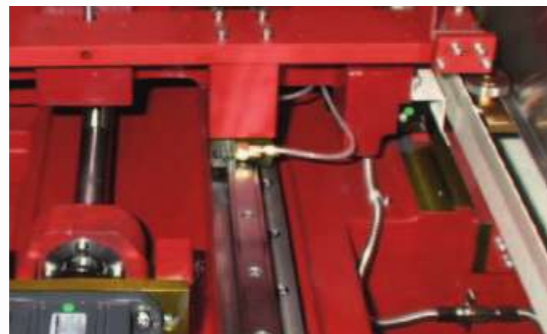
As standard, the FA-S Advance is equipped with glass scales in the X and the Y axis. These are located within the immediate vicinity of the working area for the highest precision.
