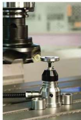
AUTOMATIC TOOL LENGTH MEASURING SYSTEM
