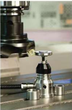
AUTOMATIC TOOL LENGTH MEASURING SYSTEM
