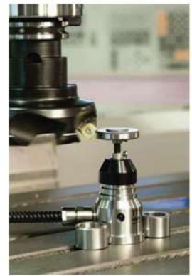
AUTOMATIC TOOL LENGTH MEASURING SYSTEM
