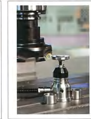
Automatic Tool Length Measuring System
