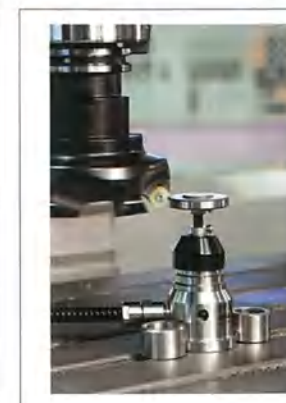
Automatic Tool Length Measuring System
