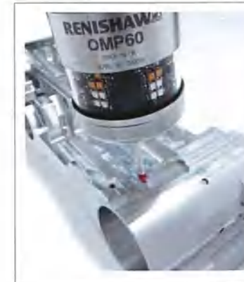
Automatic Touch Probe Centering System
