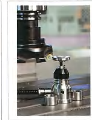
Automatic Tool Length Measuring System
