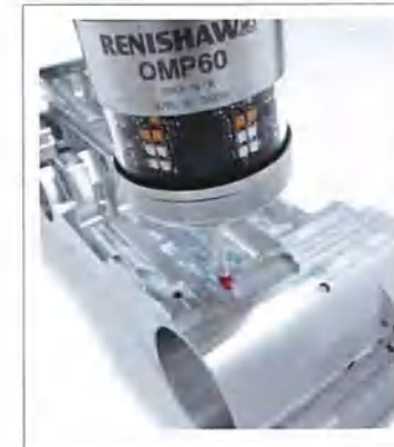
Automatic Touch Probe Centering System
