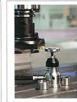
Automatic Tool Length Measuring System
