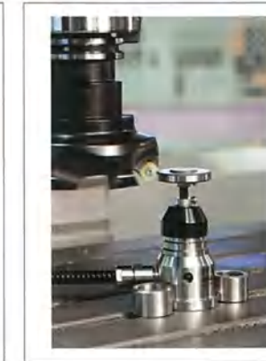
Automatic Tool Length Measuring System
