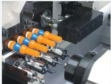
► Main & Sub-spindle simultaneous milling
