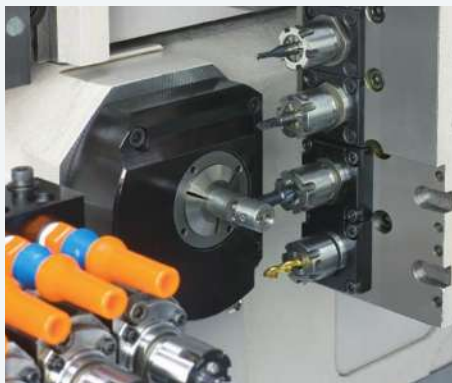
► Main & Sub-spindle simultaneous drilling and tapping
