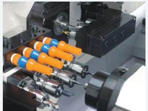
▶ Main & Sub-spindle simultaneous milling
