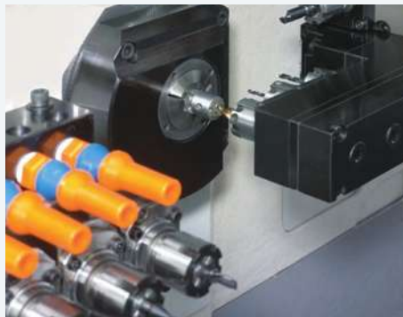
▶ Front offset drilling and tapping
