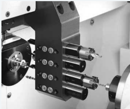
▶ Main & Sub-spindle simultaneous drilling and tapping
