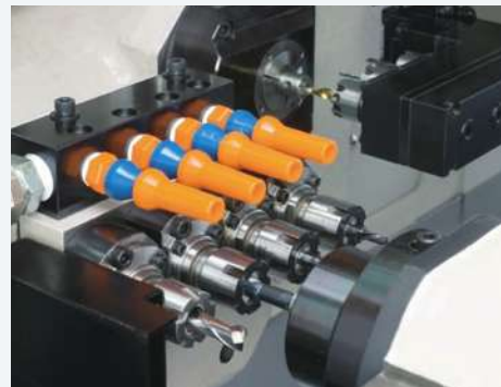
▶ Rear offset drilling and tapping
