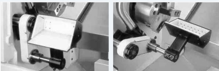
► Optional hydraulic parts catchers can be programmed to catch finished parts after cut-off. Parts conveyor systems are also available.
