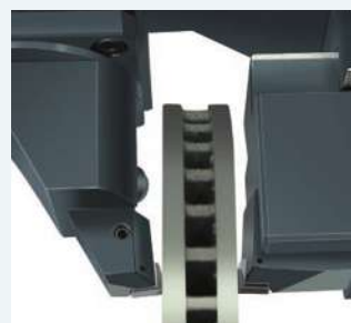
Simultaneous dual-face turning of disk brake
