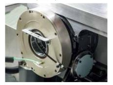
A roller gear cam is used for the tilt axis (A-axis). High retention force and a backlashless structure achieve high-speed and high-accuracy indexing.
