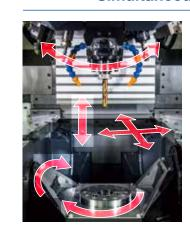
Wasted time is further reduced by positioning the X/Y/Z axes and A/C axes simultaneously with tool changes.
