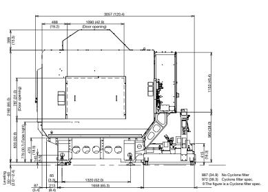
Secure 700 mm (27.6 inch) between machines as maintenance space.
