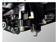
An original double plunger lock is used to secure turning tools, achieving excellent tool change repeatability.
