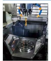
Using a fast acceleration / deceleration spindle motor and highly-responsive servo control achieves quicker starting and stopping of the spindle and turning spindle.
