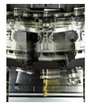
Using a compact 22-tool magazine with excellent weight balance and optimal control achieves high-speed tool change, with any wasted operation eliminated.
