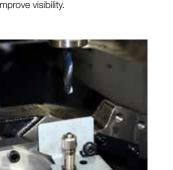
Tool breakage detector (touch type)
